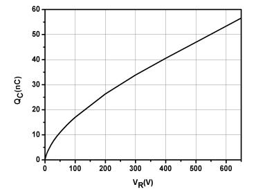
Fig.4-Total Capacitance Charge vs. Reverse Voltage
