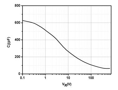
Fig.3-Capacitance vs. Reverse Voltage
