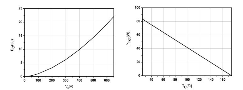
Fig.5-Capacitance Stored Energy
